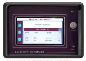
**PROGRAMMING:** The machine may be programmed for up to thirty devices per mode of operation in separate buffers. Each buffer may have up to 21 stitch bonds with individual ultrasonic power, time, force, and loop elevation control data. Program values, action prompts and fault diagnostics are displayed on a 7" LCD Capacitive Touch Screen.
