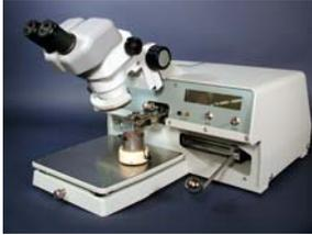
**PROGRAMMING** for three different device types may be entered into separate buffers. Each device wire may be programmed with individual ultrasonic power, time, and force (high or low) and loop elevation control data. Program values, action prompts, and fault diagnostics are exhibited on the easy to read 4 lines, 40 characters LCD sequentially with machine operation.
