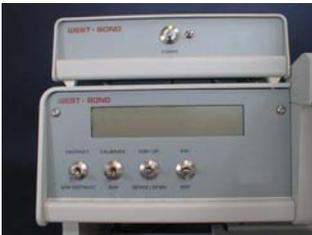
**PROGRAMMING** a device, the users can select the speed, drop of the work and data output options. Program values, action prompts, and fault codes are exhibited on the easy to read 4 lines, 40 characters LCD sequentially with machine operation. Pull Test data has a resolution of 0.1 grams with an accuracy of +/- 0.2 grams.
