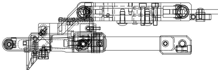
an axis located to serve both overhead and angled feed generates the clamp motions along their lines of feed action. To change between angled feed and overhead feed, it is necessary only to exchange the small clamp assemblies and to change the wire drag means. Alignment of clamps to the tool is facilitated by individual adjustments along three axes. Actuation of all clamp motion is by the same spiral cam of an inboard motor and is transferred through the pivots of the four-bar
