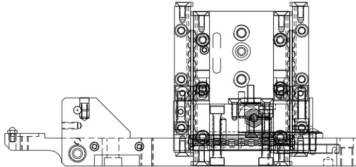
It should be understood that the pneumatic axis brakes cannot prevent deliberate efforts at movement, but that they are a significant aid in maintaining correct tool to work contact during bonding.
